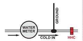
If you have a water meter, the HHC UNIT is installed on the cold water pipe, after the water meter itself, as shown. Additionally, the HHC UNIT should always be placed after any electric ground wire clamp that uses the cold water line for grounding, as shown above.
