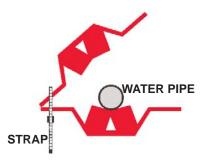
Step one: Pull strap through holes at one end of HHC unit, and loop through locking device, pulling strap almost tight.
