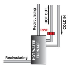
Place the HHC UNIT on the domestic hot water outlet pipe (1/2" to 3/4" pipe) as shown above. NOTE: do not place it on the heater recirculating line (1 3/4" to 2" pipe). If you are experiencing a coil blockage or restricted flow have your local plumber clean the coil.
