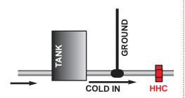
If your water is provided by a well, the HHC UNIT is installed on the cold water pipe exiting the water pressure tank. Additionally, the HHC UNIT should always be placed after any electric ground wire clamp that uses the cold water line for grounding, as shown above.
