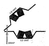
Step one- align the holes at one end of the two unit halves and insert the strap through the holes pulling the end through the fastening device on the strap. Do not tighten but leave approximately a 1 inch loop in the strap.
