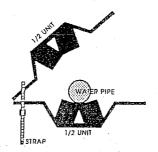
Step two-locate the place on the water pipe you are going to install the unit, Cradle the water pipe in the natural cavity of the unit, as shown above.
